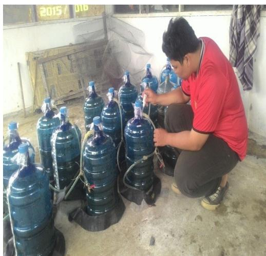
Gambar 1. Proses kontrol kualitas digester biogas
